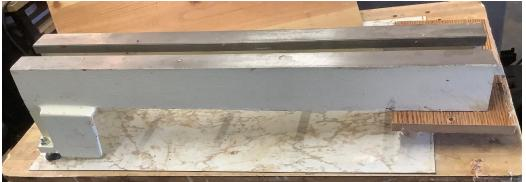
I have a 24" bed extension for a Jet Mini Lathe.
